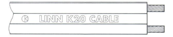
Please note that speaker cable is directional and usually provides slightly better performance when orientated in the proper direction. Linn speaker cable is imprinted with a circular Linn logo followed by the model number of the cable. When the cable is properly orientated, the circular logo will point towards the loudspeakers.
