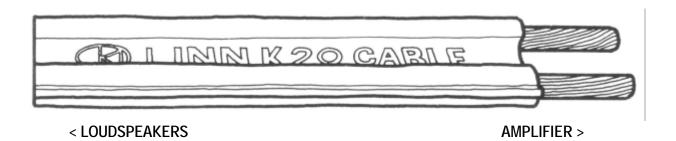
Take care to ensure that the wiring is correct. The red socket is positive and the black is negative. The positive wire (red connectors is identified by a rib along the side of the cable.
