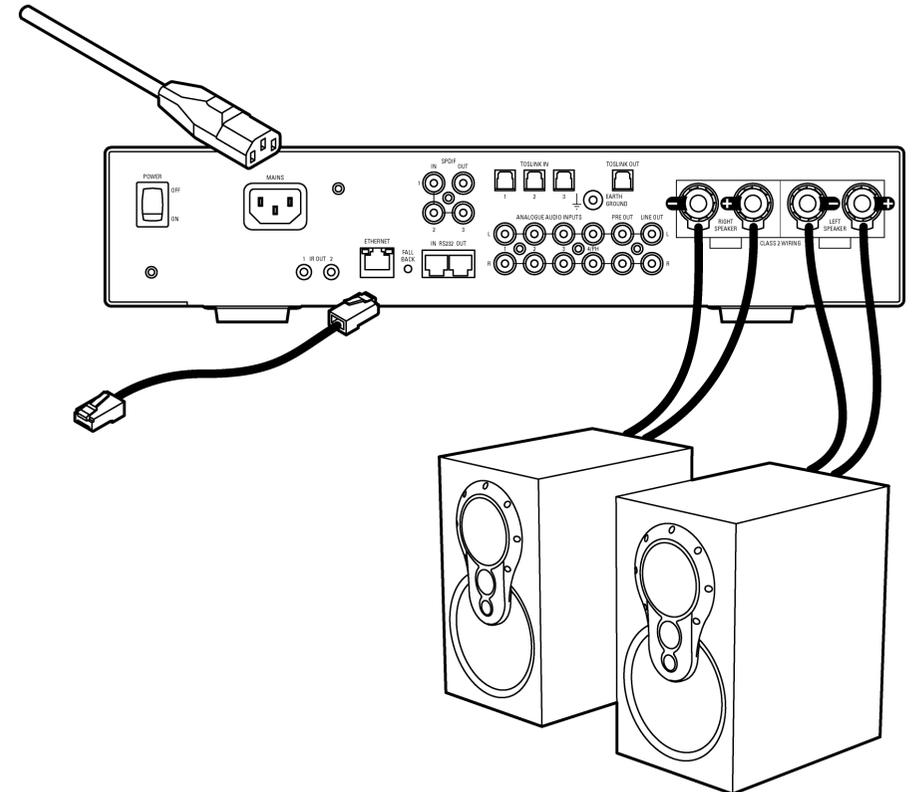
3. Connect any additional source components to the back panel using your preferred connection method (phono or balanced) - use socket **4/PH** for any turntable you wish to connect (and **do not connect** line level source components to this socket)
