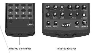
If you can see the infra-red transmitter LED on your other handset, you will be able to see when the handsets are correctly positioned after you complete the vertical and horizontal alignment steps below.
