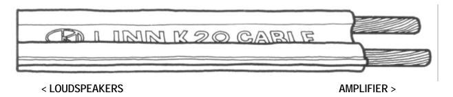
Take care to ensure that the wiring is correct. The red socket is positive and the black is negative. The positive wire (red connector) is identified by a rib along the side of the cable.
