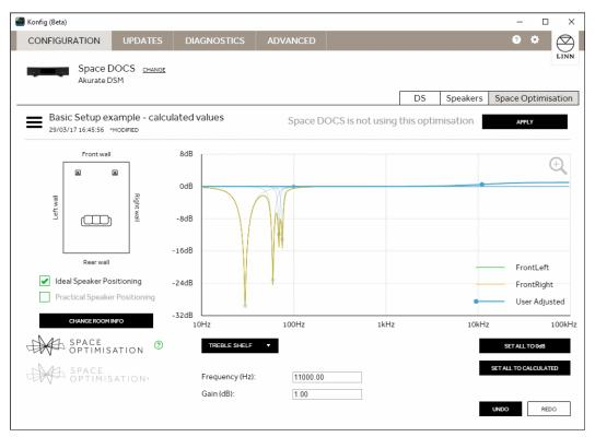
The low frequency shelf can apply cut or boost to low frequencies with a corner between 20Hz and 200Hz. The limits of cut and boost are specific to each model of speaker but typically cover the range -6dB to + 3dB. It is generally advisable when applying boost to set the corner frequency at 65Hz or lower to avoid disrupting the vocal presentation of the system.
