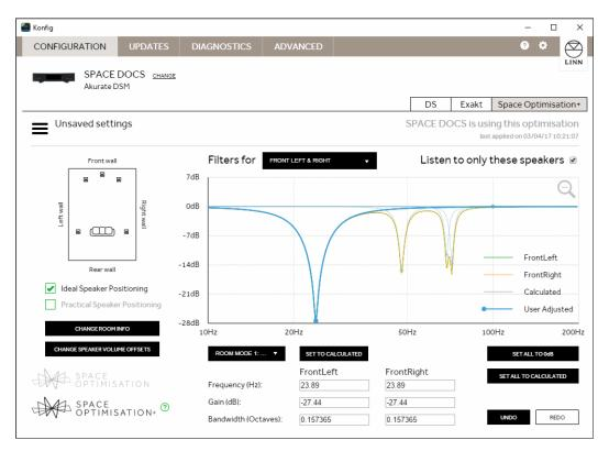
Using the process detailed in section 5.2 adjust the room mode gains frequencies and bandwidths using Tune-dem to evaluate any changes.
