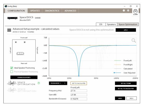
For room mode optimisation filters that are 'common' across a pair of loudspeakers the three parameters will be displayed for both loudspeakers. Any adjustments made to the filter will be applied to both loudspeakers.
