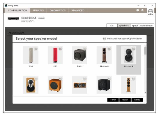
Loudspeakers which have been measured for Space Optimisation by Linn are indicated by a symbol in the top right corner. If your loudspeaker model is not selectable you should select 'Other' from the end of the list. Any model which has yet to be measured will raise the message below:
