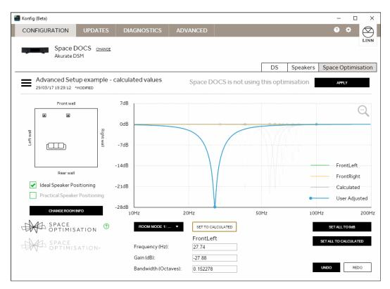
Using the Tune-dem re-instate each filter in turn, always starting with the lowest frequency, and ensure that each optimisation filter improves the musicality of the system. If re-instating a filter has no audible effect then return the filter's gain to zero and move to the next filter
