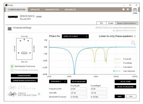
Changing the selection in the 'Filters for' drop down list switches between common channels within the surround system. When a channel is selected the graph and associated controls will change to reflect the optimisation applied to the displayed channels.
