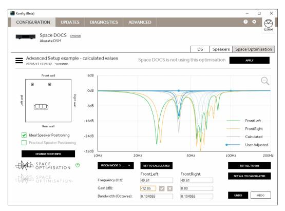
The left filter gain can continue being increased until it also reaches 0 dB with no further effect on the right filter gain.
