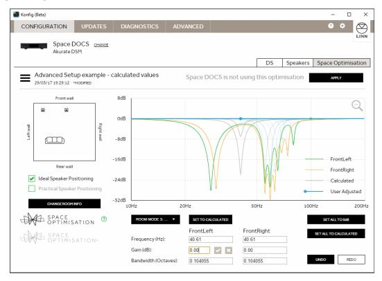
With both filter gains set to 0 dB, a decrease of 1 dB to the right filter gain results in the left speaker gain setting itself to -15.89 dB. Konfig has re-applied the gain difference of 14.89 dB.
