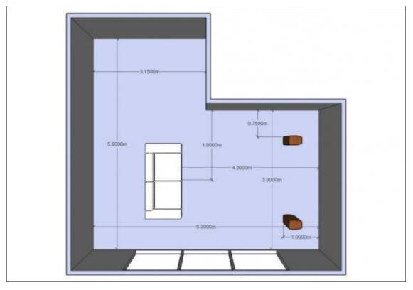
For this example, the loudspeakers are placed on the right side across the 3.9m width firing along the 6.3m length of the room. The initial rectangular layout would have a length of 6.3m and a width of 3.9m.
