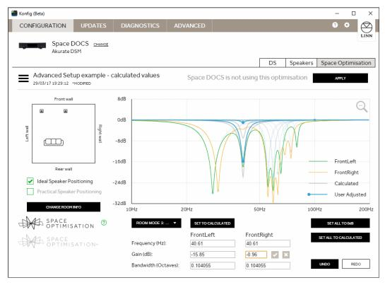
Adjusting the left speaker by a further 3 dB now gives a left filter gain of -12.85 dB, but a right filter gain of 0 dB.
