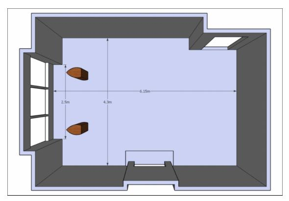
As the bay window along with the remainder of the front wall forms a staggered surface some smearing of room modes relating to the length of the room may occur. This can be countered by slightly increasing the bandwidth of any length modes.
