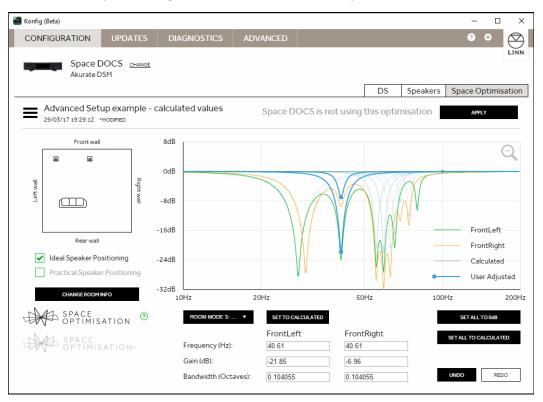
For 'ROOM MODE 3' the left and right filters show a gain difference on 14.89 dB. Increasing the gain of either speaker by 6 dB results in a left filter gain of -15.85 dB and a right filter gain of -0.96 dB. The 14.89 dB difference is maintained.
