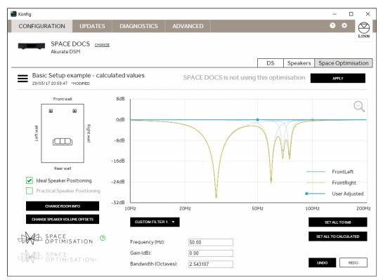
The parameters applied to define a custom filters may be derived by trial and error and Tune-dem or by information captured by a third party measurement system. As with the bass and treble shelf filters positive gain can be applied when using a custom filter. This is limited to 2 dB to avoid risk of damage to the attached loudspeakers.
