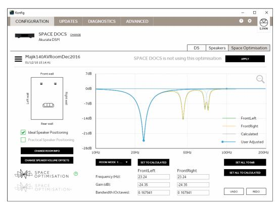
DO NOT enter the room set-up ('CHANGE ROOM INFO'), DO NOT press 'OPTIMISE'. Doing so will replace the imported mode filters with a newly calculated set of optimisation filters based on the new optimisation algorithm.
