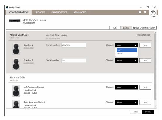
If your loudspeakers contain integrated Exakt amplifier modules this page will automatically populate. You will need to assign the speakers to left and right.
