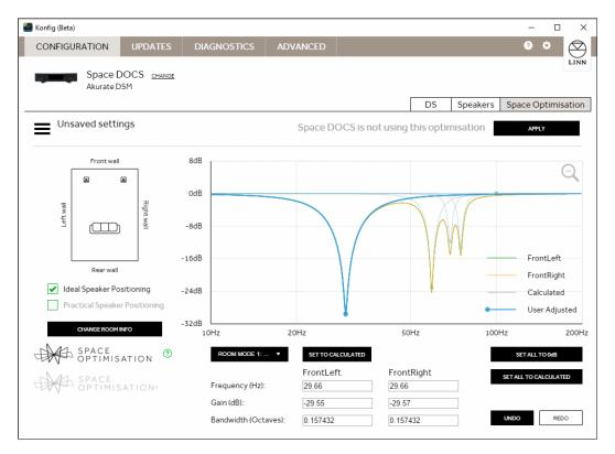
Konfig will now calculate the optimisation filters for room modes and loudspeaker placement (if practical placement has been entered for the loudspeakers). Once calculated the screen will change to show the result of the room mode optimisation algorithm.
