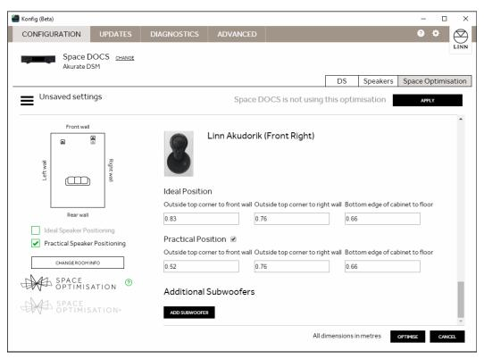
Check the 'Practical Position' tick-box and enter new distances into Konfig. Repeat for the right loudspeaker.
