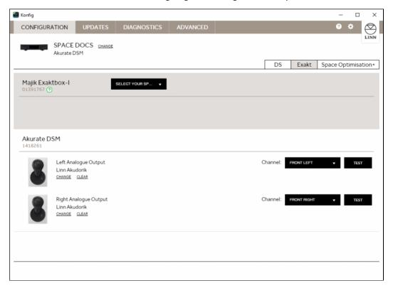
De-select the speakers assigned to the analogue channels by clicking on 'CLEAR' for both left and right speakers.
