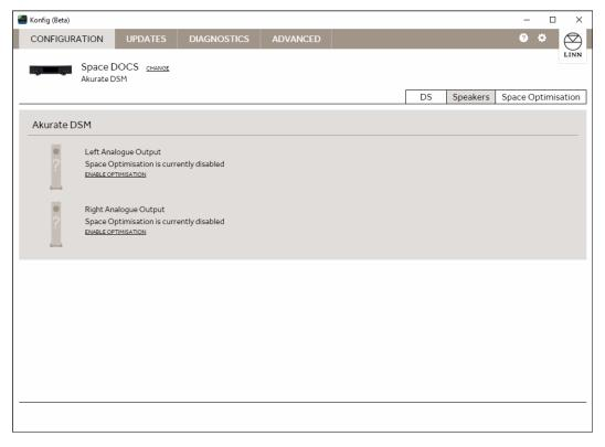
The speakers will automatically assign channels 'LEFT' and 'RIGHT', click 'APPLY' and after a moment you will see the message 'Updates successfully applied'.
