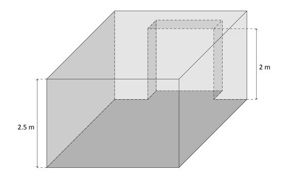
Consider a wall with a large recess of height equal to 50% of the room height, as shown below; the recess should here be incorporated into the floor plan, with a depth given by the half of the maximum recess depth.
