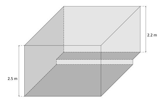
Consider a stepped floor with two equal-area sections, as shown below; the average height measurement here would be the standard average height, 2.35 m.
