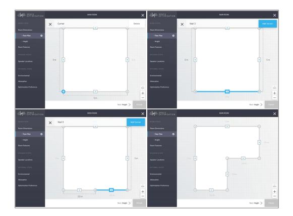
Once your floor plan has been defined click on the **Next: Height** > link in the bottom navigation pane to enter the **Height** step, as shown below. Note that rooms with non-flat floors or ceilings are currently unsupported, and so a room simplification procedure must be adopted, as outlined in §3.4. Enter the height of your room and click on the **Next: Room Features** > link in the bottom navigation pane.
