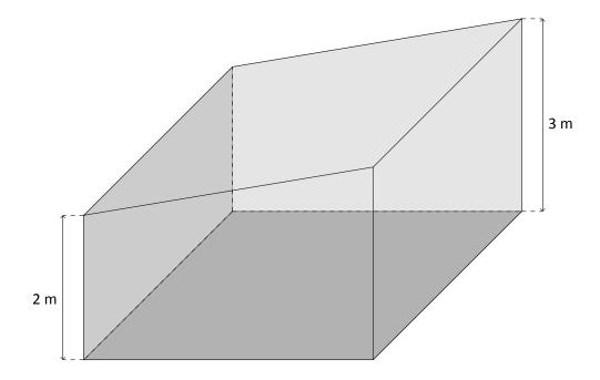
Consider a pitched ceiling, as shown below; the average height measurement here would be 2.33 m.
