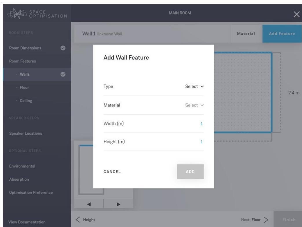
Once a feature has been added to the wall, as shown below, you can select it with a click and drag it to any desired location or enter the measurements in the contextual control bar at the top, switching between the
