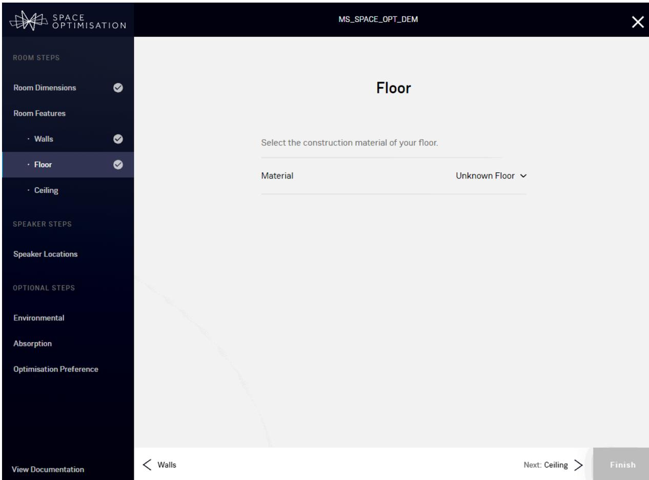
**Unknown Floor** provides an averaged absorption coefficient which should be used when the construction material is unknown. Note that floor features are currently unsupported, and so an approximation procedure must be adopted, as outlined in §3.2.1.
