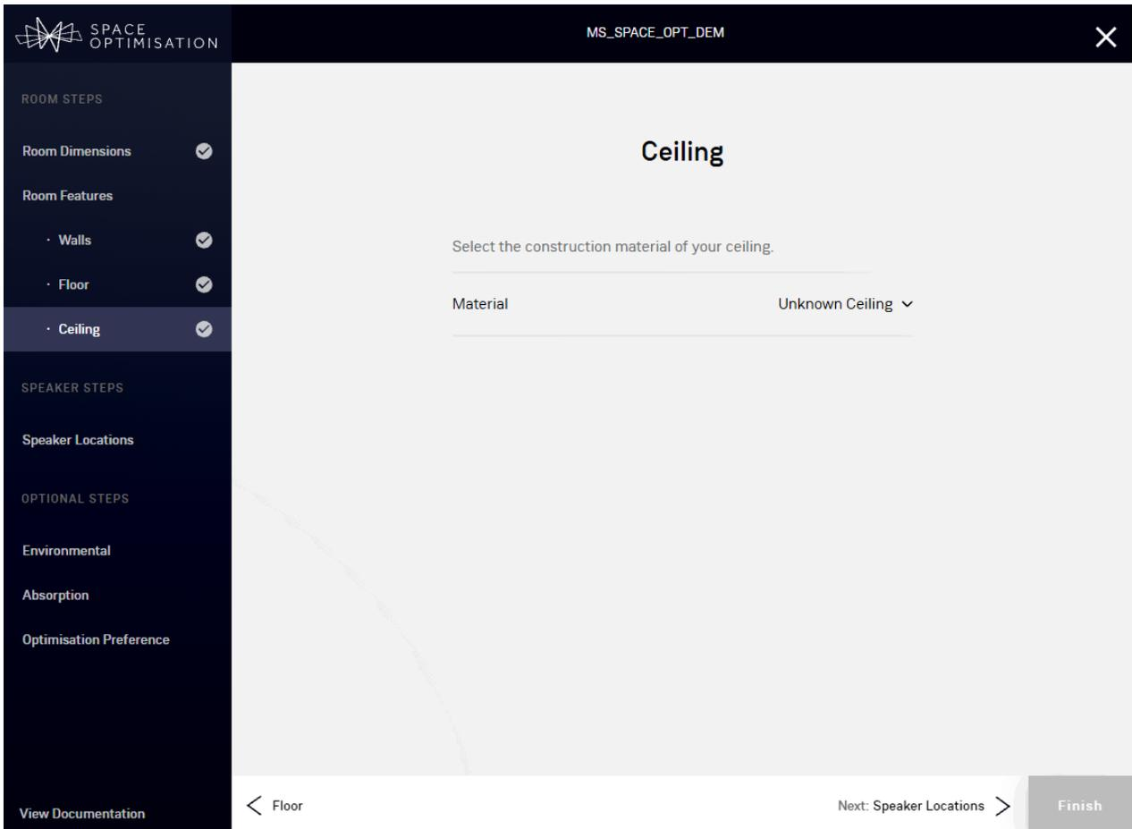
**Unknown Ceiling** provides an averaged absorption coefficient which should be used when the construction material is unknown. Note that ceiling features are currently unsupported, and so an approximation procedure must be adopted, as outlined in §3.2.1.
