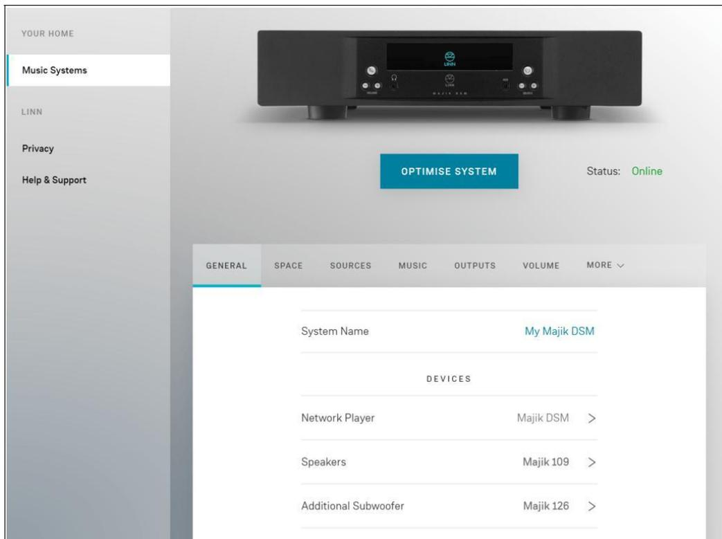
You may also add multiple additional subwoofers to your music system; each additional subwoofer will then be listed under the **General** tab, as shown below; note that you can change the assigned channel of an additional subwoofer at any time by clicking on the additional subwoofer's name under the **General** tab and reassigning the channel using the **Channel** drop-down menu or remove it by clicking on the **Remove Additional Subwoofer** button.
