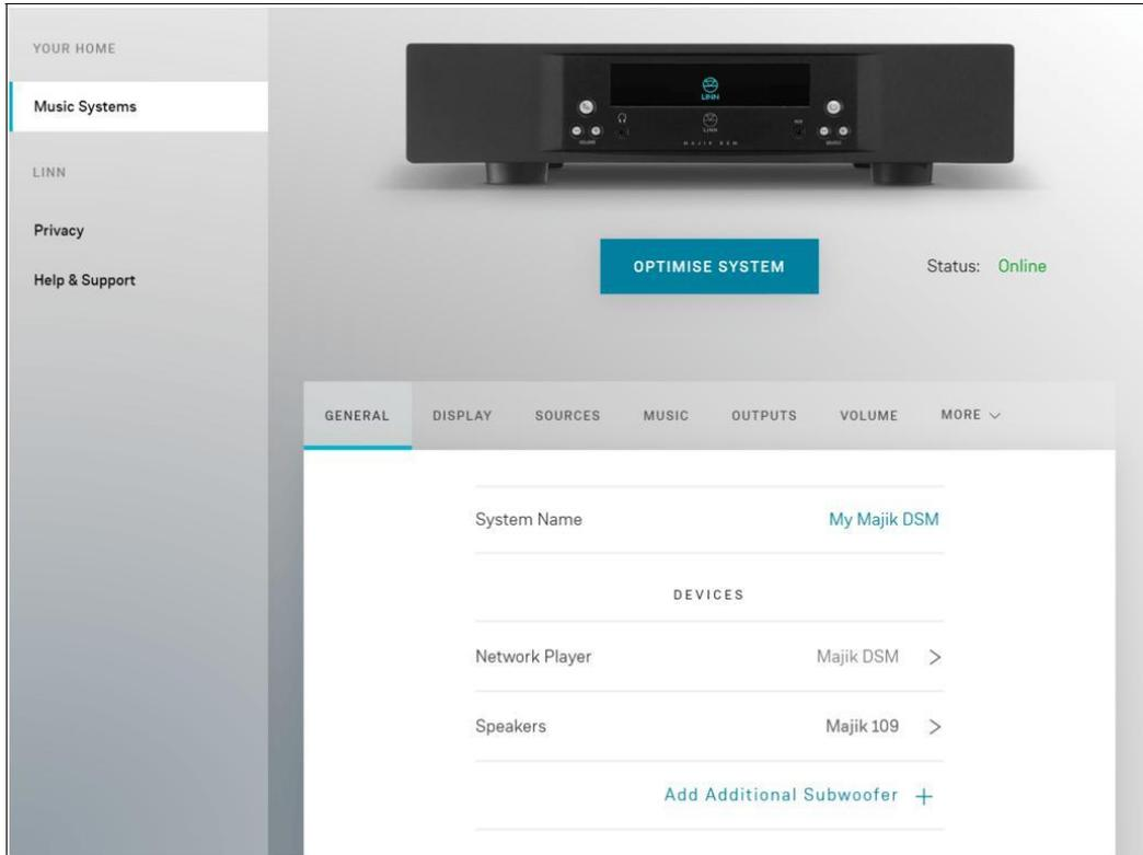
Click on the **Add Additional Subwoofer** link; a dialog prompting you to provide the channel, manufacturer and model of your additional subwoofer will appear, as shown below. Select the channel, manufacturer and model of your additional subwoofer using the drop-down menus, then click on the **Add** button; if your additional subwoofer's manufacturer or model does not appear in the drop-down menu, select **Other**.
