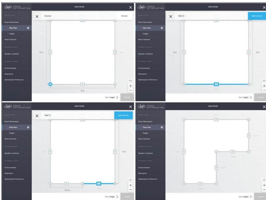
Once your floor plan has been defined click on the **Next: Height** > link in the bottom navigation pane to enter the **Height** stage, as shown below; note that rooms with non-flat ceilings or floors are currently unsupported, and so a room simplification procedure must be adopted, as outlined in §3.4. Enter the height of your room and click on the **Next: Room Features** > link in the bottom navigation pane.
