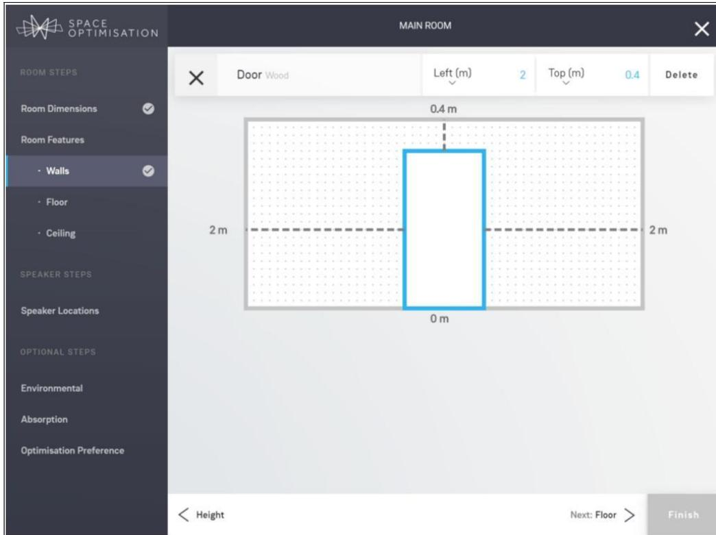
Once the construction material and features have been defined for all your walls click on the **Next: Floor >** link in the bottom navigation pane to enter the **Floor** stage, as shown below. Select the construction material using the **Material** drop-down menu: **Concrete** describes any solid or heavy construction, including concrete or stone; **Suspended Floor** describes any suspended construction, including suspended floorboards.
