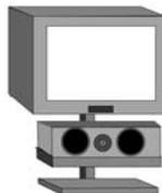
The TRIKAN can be positioned above or below a television set. The TRIKAN is magnetically screened, so it will not affect the television picture.
