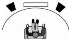
The TRIKAN should be placed slightly closer to the rear wall than the main left and right speakers. The distance from the listener to each speaker should be the same.
