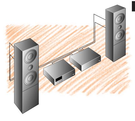
For more performance, you can use two or three LK85/140s to bi-amp or tri-amp to the loudspeakers, each amplifier driving the bass, midrange, and treble signals separately.
