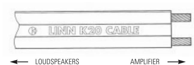
Take care to observe the correct polarity. The red socket is positive and the black is negative. The positive wire is identified by a rib along the side of the cable.
