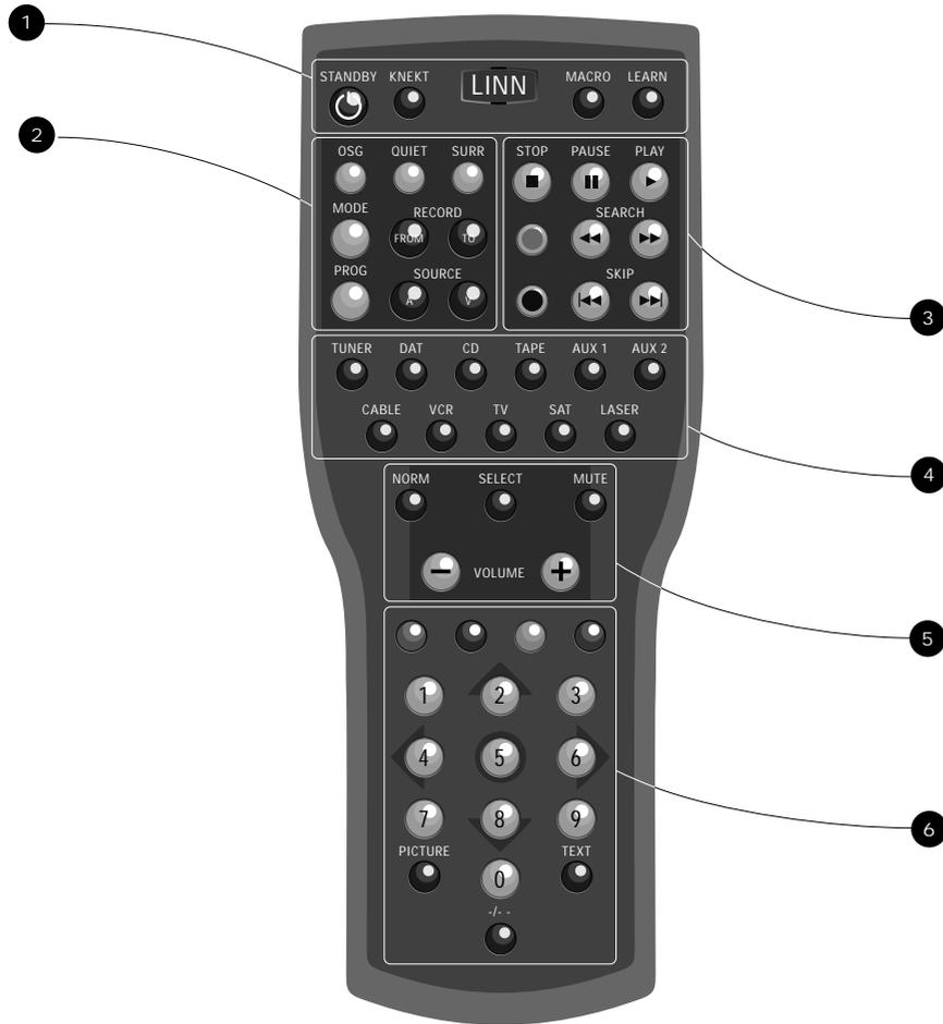
1. STANDBY Switches the unit to standby, or switches it on from standby.
