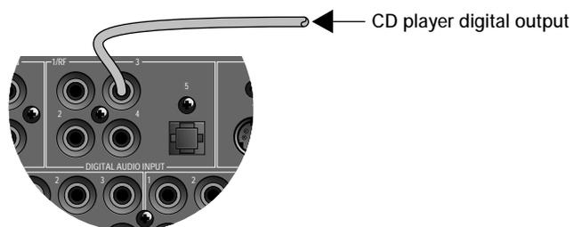
Alternatively if the CD player provides an optical output you can connect this to the System Controller's DIGITAL AUDIO INPUT 5, using an optical cable.
