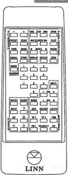
The MAJIK-I is supplied with a standard handset which controls the amplifier and provides basic control for other Linn source components and the Linn KAIRN. The larger handset supplied with other Linn products may also be used with the MAJIK-I.
