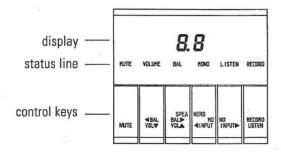
Although there are many sophisticated features, all commonly used functions require only one key press. To access the less commonly used functions, such as balance, two keys must be pressed at the same time. The status of the MAJIK-I is always indicated through the row of indicator lights.
