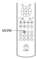
When listening to a station on the FM or AM band you can view the station's frequency on the display by pressing the MORE key. Press **MORE** again to return to the previous view.
