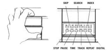
KARIK OPERATION Operating the KARIK with the remote control provides the most efficient method of accessing the functions, and you will probably use this method on a day-to-day basis. Manual operation of the KARIK, using the buttons on the control area, is described below.
