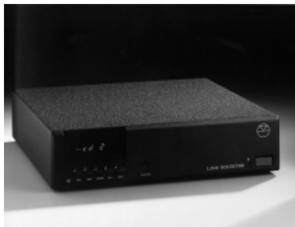
Ten clear solid-state paths for music. Micro-processor control of multiple inputs and RS232 connectivity
