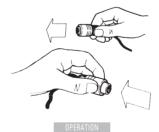
The switch on the LP12 provides a trigger to the electronics to start, stop or change the speed of the motor. It does not break any mains connection. The power switch on the LINGO power supply isolates mains. However, to prevent electric shock, never remove the bottom cover from the turntable with the LINGO connected, or the case from the LINGO power supply while it is connected to the mains.
