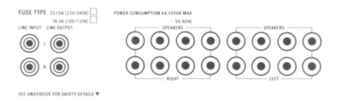
If you have speakers that allow passive bi-amplification or tri-amplification (or if you are using multiple LK100s to drive several sets of speakers), the signal from the pre-amplifier is routed to the **LINE INPUT** sockets of the first LK100. The signal is then chained to the second LK100 by connecting an RCA phono interconnect cable from the **LINE OUTPUT** of the first LK100 to the **LINE INPUT** sockets of the second 1K100. This connection procedure is repeated for each LK100 in the chain.
