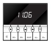
Press the power button on the front panel. The time will appear on the display whenever power is applied.
