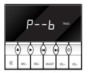
Load a disc and press **OPEN**. Wait until the display shows the disc time then the number of tracks. Press and hold **DISPLAY** for two seconds. To start again press **OPEN**.
