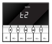
Press **TP2** on handset to toggle between the source of the recording and the recording destination.
