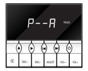
Load a disc and press **OPEN**. Wait until the display shows the disc time then the number of tracks. Press and hold **DISPLAY** for one second. Holding for longer will enter programme mode B. To start again press **OPEN**.
