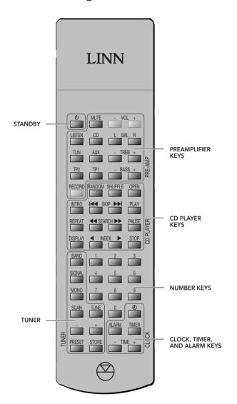
The CLASSIK is supplied with a remote control handset which provides access to all of the functions available from the front panel. In addition it provides several more advanced features, including selecting tracks by number and programming a selection of tracks.
