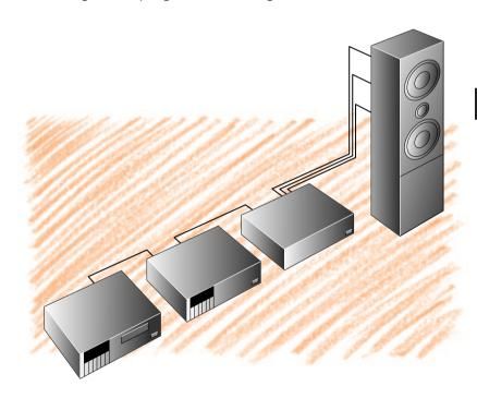
To further enhance performance, you can use two or three LK240s to bi-amp or tri-amp to the loudspeakers, each LK240 driving the bass, midrange, and treble signals separately.
