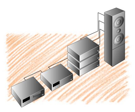
When bi-amping or tri-amping the highest possible performance can be obtained by removing the passive crossover units from the loudspeaker and fitting active crossover modules to the LK240 to accurately divide the signal into the appropriate frequency bands. This is known as active playback.
