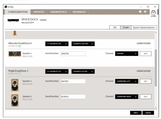
If you have previously used the analogue outputs from DSM ensure that these are deselected. Scroll to the bottom of the screen to see the analogue outputs. If these have an assigned speaker click on 'CLEAR' for each of the analogue outputs and click on the **'APPLY'** button.
