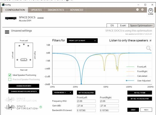
Using the process detailed in <u>section 5.2</u> adjust the room mode gains frequencies and bandwidths using Tune-dem to evaluate any changes.
