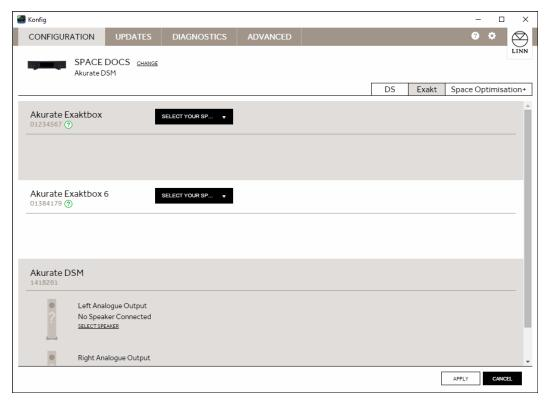
If the system contains integrated Exakt loudspeakers Konfig will populate them automatically into the list. Any Exaktboxes will need to be configured manually. Once you have selected any speakers connected to your Exaktbox all speakers require to be assigned by channel in the surround system.
