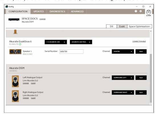
If you are using a mixed Exakt and analogue system, assign the Exakt speakers and select the appropriate channels for the analogue output channels. Click on the 'APPLY' button.
