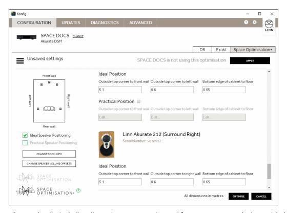
When all room details, including dimensions, construction and features are entered, along with the listening position and locations of all speakers in the multi-channel set-up, click the 'OPTIMISE' button. After a moment you will see the Space Optimisation+ screen. Click 'APPLY' to apply the optimisation.
