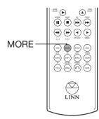
When listening to a station on the FM or AM band you can view the station's frequency on the display by pressing the **MORE** key. Press MORE again to return to the previous view.
