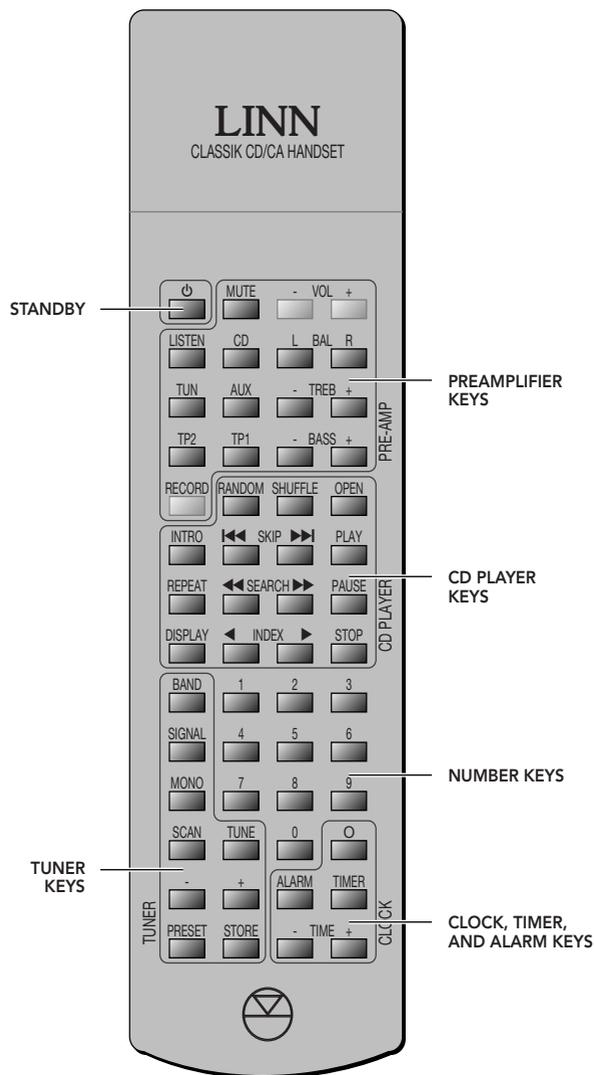
The IKEMI and GENKI are supplied with a remote control handset which provides access to all of the functions available from the front panel. In addition it provides several more advanced features, including selecting tracks by number and programming a selection of tracks.
