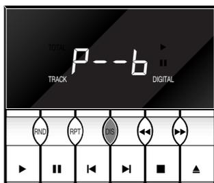
Load a disc and press **OPEN**. Wait until the display shows the disc time then the number of tracks. Press and hold **DIS (DISPLAY)** for two seconds. To start again press **OPEN**.
