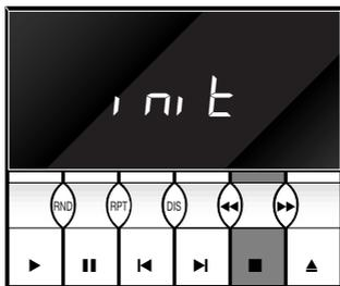
Factory default settings (initialise). Switch the power on while holding the **STOP** button, for ten seconds.
