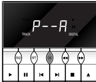
Load a disc and press **OPEN**. Wait until the display shows the disc time then the number of tracks. Press and hold **DIS (DISPLAY)** for one second. Holding for longer will enter programme mode B. To start again press **OPEN**.
