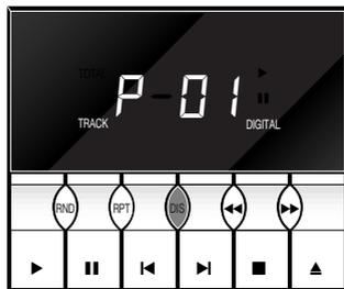
Press **DIS (DISPLAY)** to save this programme step. Using **SKIP** or the handset repeat for all chosen tracks then press **PLAY**.
