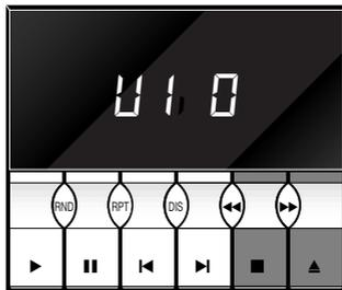
User Options. To customise the operation of the **IKEMI** and **GENKI** go to the User Options mode. Switch the power on while holding the **OPEN** button for twelve seconds. **OPEN** selects the Option, **STOP** changes its value. See the following table for the options. To exit press and hold **OPEN** for five seconds.
