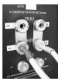
**<u>BI-WIRING</u>** Remove both linking plates. Leave the bottom two sockets unused.
